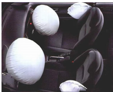
Deployed driver and passenger airbag modules and side impact cushions
